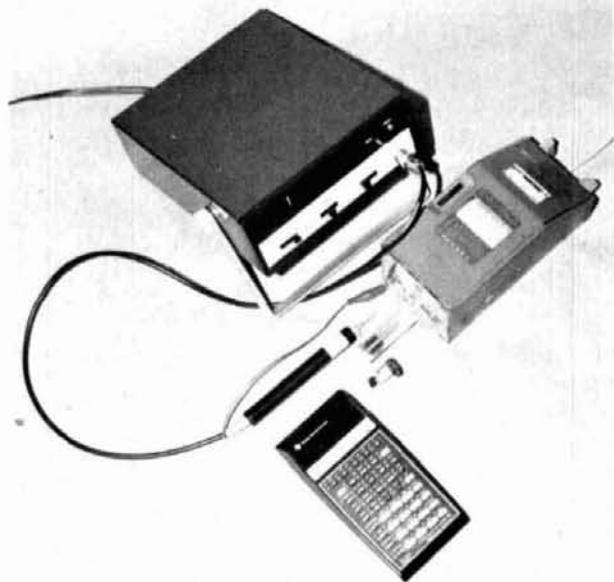
fig. 5. Setup used to speed up the inductance measurement process. The toroidal coil under test was paralleled by a known precision silver mica capacitor. The exact frequency of the circuit was read with a digital counter which measured the frequency of rf generated by the grid dip meter at resonance. All numbers were inputted to the TI-59 programmable calculator which resolved the equation for L or C.
